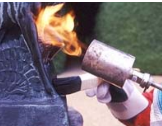
Flame heating a surface of bronze before microcrystalline wax is applied to hot metal, at Anglesey Abbey, Cambridgeshire.
