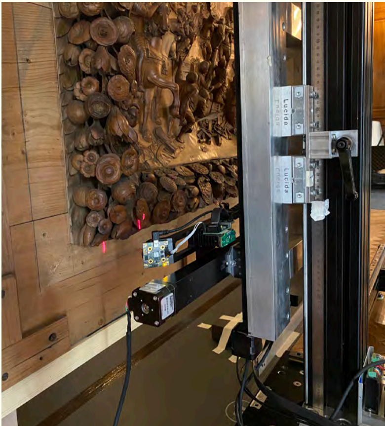
4. Factum Foundation undertaking 3D scanning of The Crucifixion (NT 931239) at Dunham Massey, Cheshire Photo: National Trust/Emma Campagnaro
